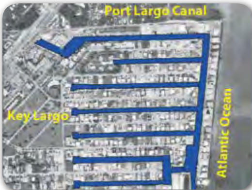
Port Largo Canal is a long, dead-end canal system with poor flushing. Canals were created by dredging and filling mangrove shorelines to create “fastland” for residential development.
