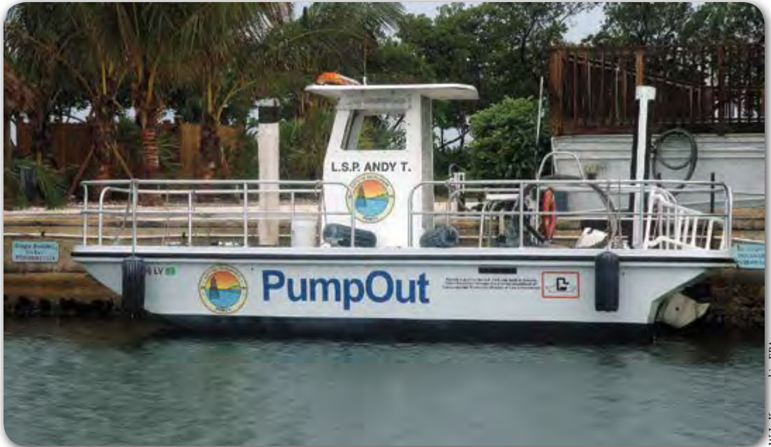
Pump-out facilities removed 99,000 gallons of vessel sewage during the first year of operation in Boot Key Harbor. Before the no-discharge zone designation, sewage would have been discharged directly to surface waters.
