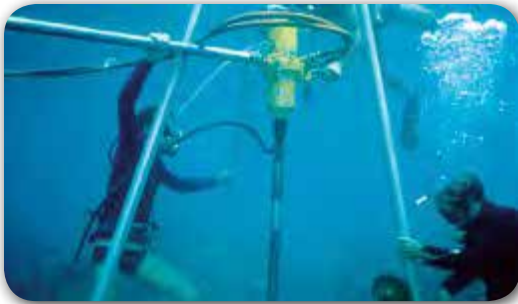
Scientists use a pneumatically powered coring device to obtain coral cores.
