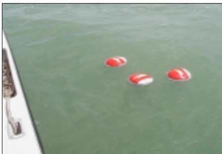
Shallow water drifters deployed for testing in Whipray Basin are anticipated to greatly assist scientists in their efforts to map the dynamics of water movement in Florida Bay.
